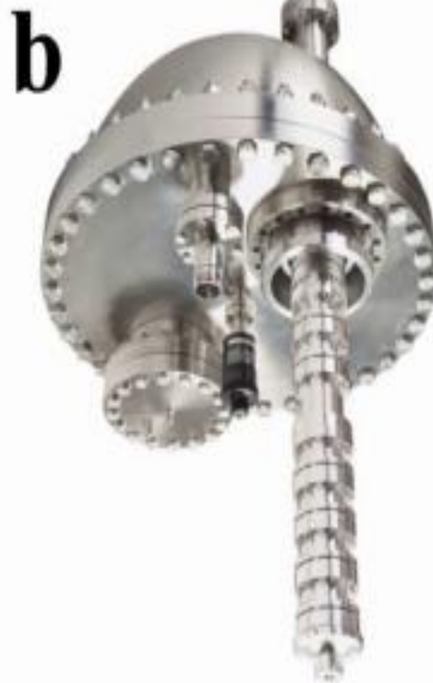
Figure 2.26. Scheme (a) and picture (b) of hemispherical electrons analyzer for XPS. Dotted lines in the scheme represent electron path.
